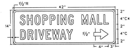
D-70S 42" X 14" Letters - White Refl. Symbol - White Refl. Border - White Refl. Background - Blue Refl.
